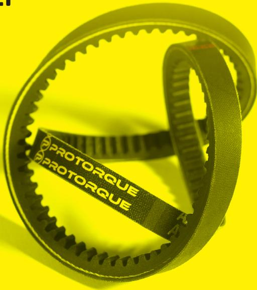
Universal classical profile coupled with a cogged cushion allows for increased belt flexibility and improved longer lasting performance, when compared to wrapped belts. Lower depth allows effective running on smaller diameter pulleys.
